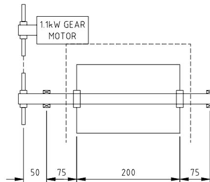
The forces are oriented in the vertical, including the drive sprocket force. This arrangement produces the highest loads on the shaft. The gearbox can be oriented in the horizontal. Such an arrangement would not have vertical loads at the sprocket. The sprocket load would then be at 90 degrees to the belt tension. This would produce less overall stress in the shaft and a smaller shaft could be used. However in this design the worst-case orientation will be used.
